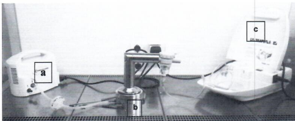
Fig. 1 System set up – deposition on stainless steel disks. a: vacuum pump, b: Andersen cascade impactor, c: Philips nebuliser
